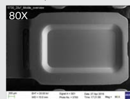
LED Leadframe with Silverjet HS-2000 Silver Deposit
