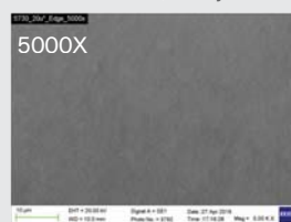
LED Leadframe with Silverjet HS-2000 Silver Deposit
